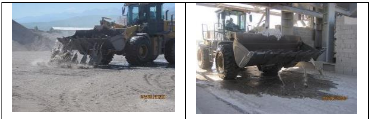
Figure 43 Watering of the production site with flushing water.
